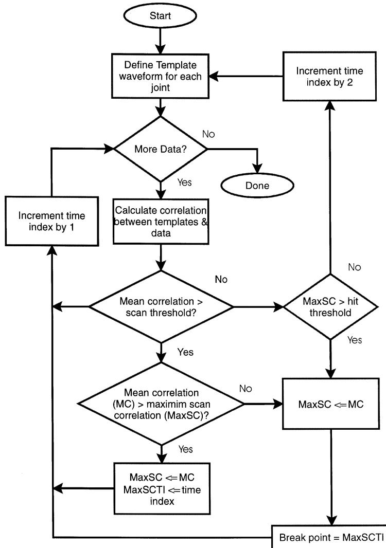
Fig. 1. Flow chart diagram of template matching algorithm.
