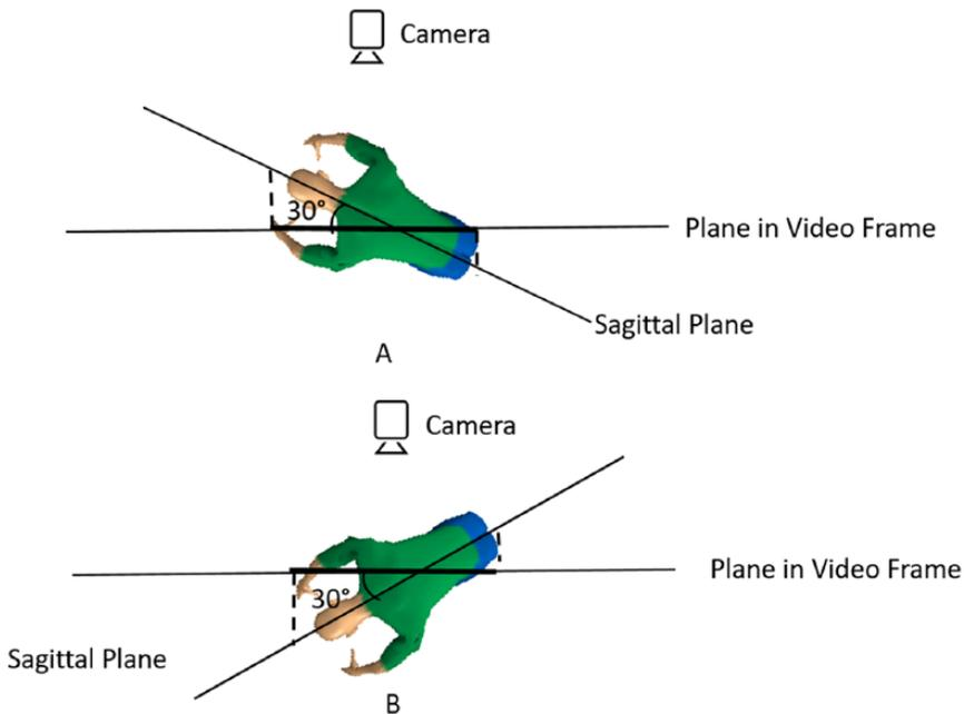
Figure 7. Demonstration of bounding box width as the projection of the mannequin's sagittal plane length on the plane on video frame, and the bounding box widths are identical for when the mannequin is rotated (A) counterclockwise and (B) clockwise.
