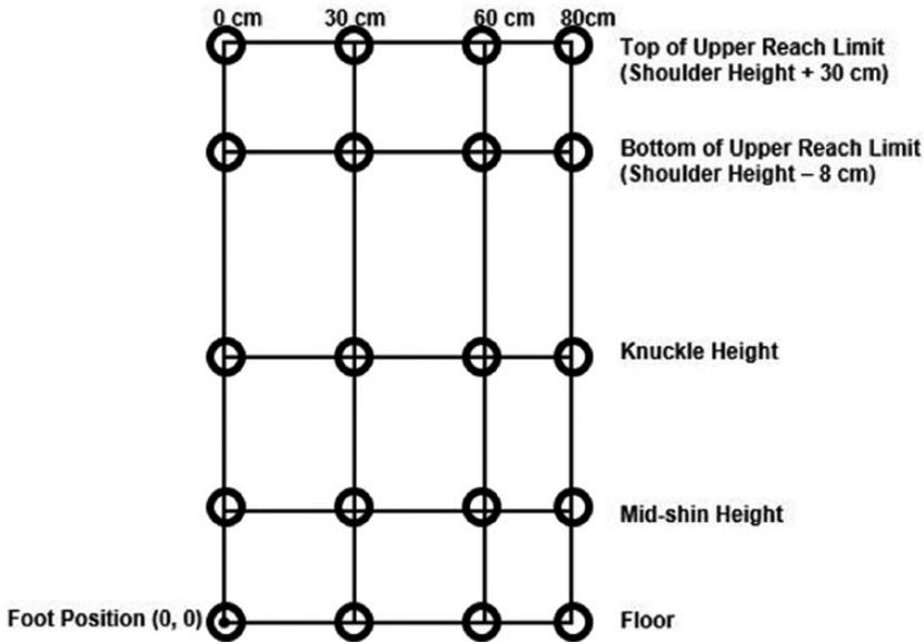
Figure 5. Representation of intercepts of three horizontal and four vertical zones.
