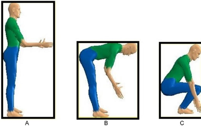
Figure 2. Examples from 3DSSPP of (A) standard standing, (B) stoop, and (C) squat lifts and their associated bounding box dimensions.
