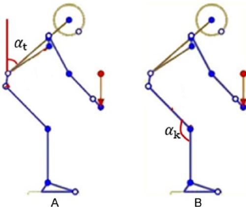
Figure 3. 3DSSPP models demonstrating (A) torso angle ( $\alpha_t$ ) and (B) knee angle ( $\alpha_k$ ) measured to classify lifting postures.
