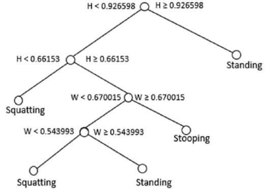
*Figure 8.* Decision tree generated from training data set, where H is the bounding box height normalized by standing height and W is the bounding box width normalized by standing height.
