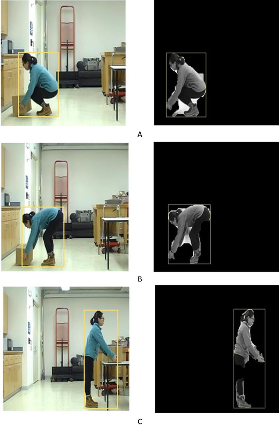
*Figure 1.* (Left) Original video frames and (right) background subtracted computer vision images of a subject performing (A) squatting, (B) stooping, and (C) standing lifts during a lab-simulated task. In the task, the subject picks up an object from the shelf on the left of the video frame, transfers and lowers it, and places it on the ground in the right portion of the video frame. A rectangular bounding box encloses the subject in each image, independent of the object lifted.
