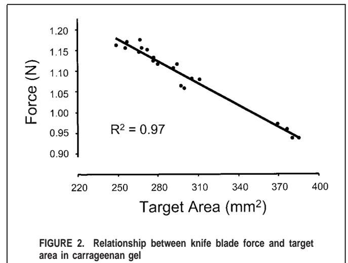
FIGURE 2. Relationship between knife blade force and target area in carrageenan gel
