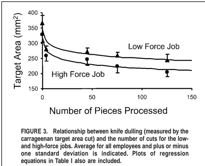
**FIGURE 3.** Relationship between knife dulling (measured by the carrageenan target area cut) and the number of cuts for the low- and high-force jobs. Average for all employees and plus or minus one standard deviation is indicated. Plots of regression equations in Table I also are included.
