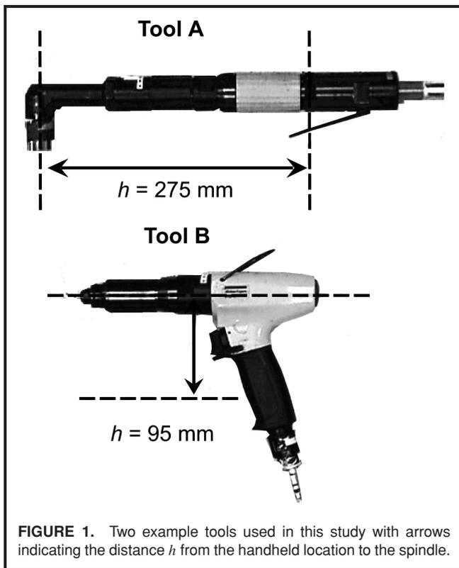
**FIGURE 1.** Two example tools used in this study with arrows indicating the distance  $h$  from the handheld location to the spindle.
