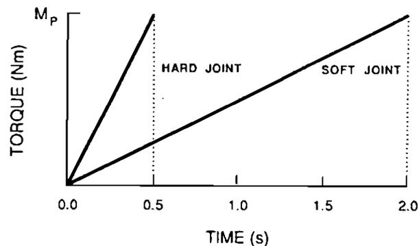
Figure 2. Template for spindle torque output during torque build-up phase. Torque build-up time for both soft joints and hard joints are illustrated.  $M_p$  is the peak spindle torque which is the desired torque output and is independent of joint stiffness.
