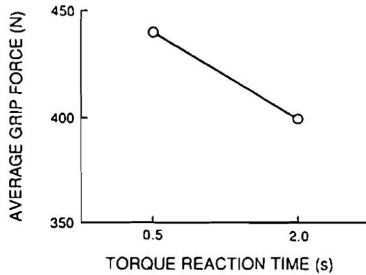
Figure 6. Average grip forces during the Torque Reaction phase for long and short torque reaction times (five subjects).
