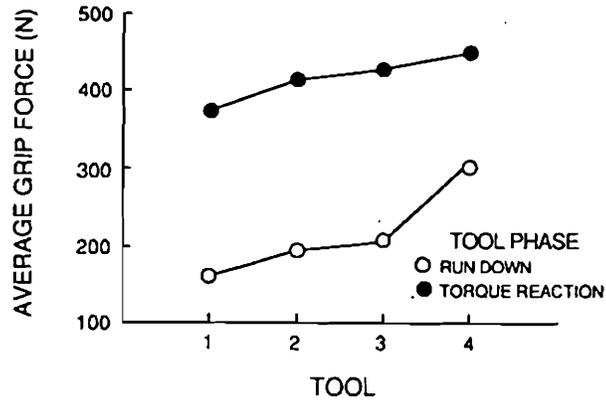
Figure 5. Average grip force vs. Tool for the Run-down and Torque Reaction phases (five subjects).
