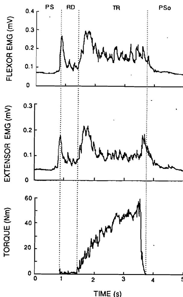
Figure 3. Representative nutrunner spindle torque output and associated forearm flexor and extensor rms EMG response for a 2 s long torque reaction time. The Pre-start phase is indicated by PS, the Run-down phase is indicated by RD, the Torque-reaction phase is indicated by TR, and the Post Shut-off phase is indicated by PSo.
