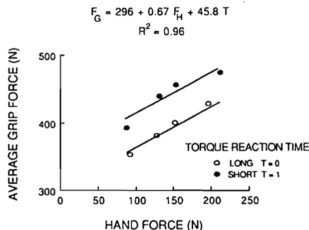
Figure 8. Average grip force ( $F_G$ ) during the Torque Reaction phase for both short and long torque reaction times plotted against average peak hand force ( $F_H$ ) for five subjects. Regression lines are included. The indicator variable ( $T$ ) was equal to zero for the long torque reaction time and equal to one for the short torque reaction time condition.
