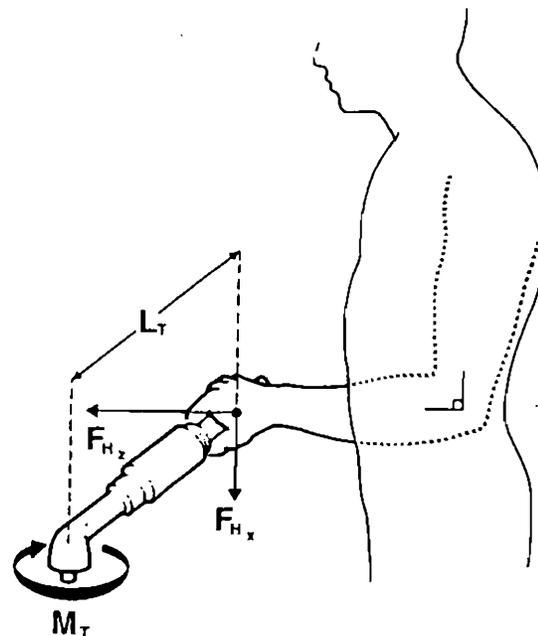
Figure 1. Forces and moments produced during right angle nutrunner operation acting against the hand. The coordinates are based on the International Organization for Standardization (ISO 1984) hand and arm basiocentric coordinate system, referenced with respect to the handle and hand.
