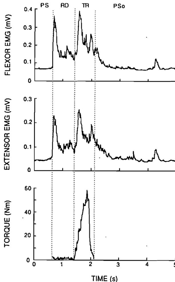
Figure 4. Representative nutrunner spindle torque output and associated forearm flexor and extensor rms EMG response for a 0.5 s short torque reaction time. The Pre-start phase is indicated by PS, the Run-down phase is indicated by RD, the Torque-reaction phase is indicated by TR, and the Post Shut-off phase is indicated by PSo.
