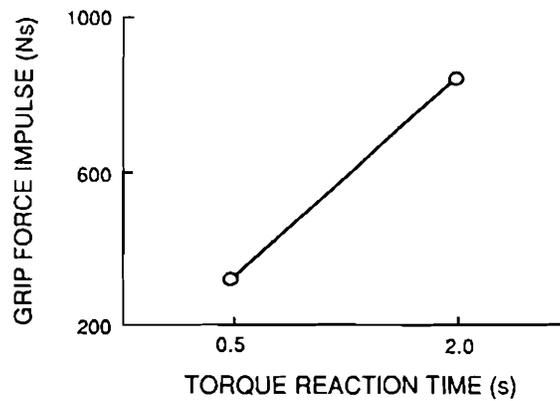
Figure 7. Average grip force impulse during the Torque Reaction phase derived from integrating rms EMG records scaled for grip force, for long and short torque reaction times (five subjects).
