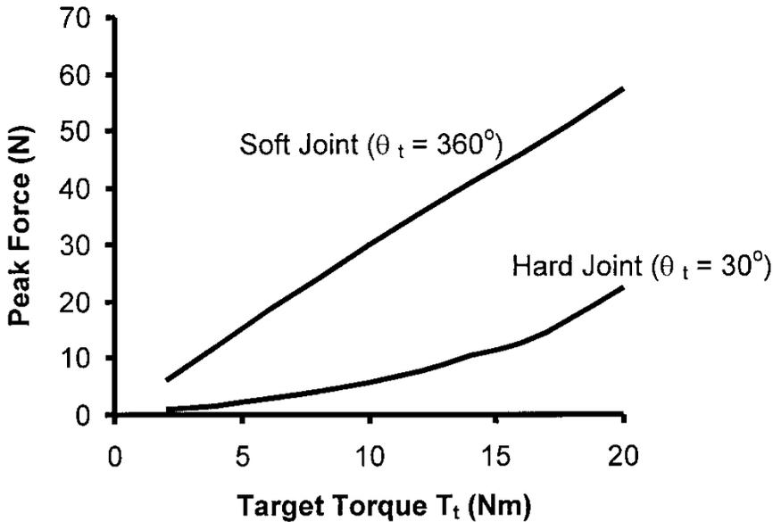
Figure 9. Plots of target torque vs. predicted handle force for two threaded fastener joint rates using a right angle tool ( $W = 2.27$  kgw,  $I_{tool} = 0.001457$  kg·m<sup>2</sup>,  $T_{max} = 25$  N,  $S_0 = 366$  rpm,  $L_{ly} = 34.5$  cm). Parameters used for the calculation are from Lin (2001):  $J_{subject} = 0.299$  kg·m<sup>2</sup>,  $k_{subject} = 283.6$  Nm/rad,  $c_{subject} = 5.95$  N·m·sec/rad.
