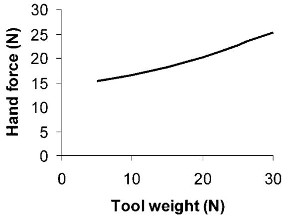
Figure 6. Handle force vs. tool weight in tool operation.
