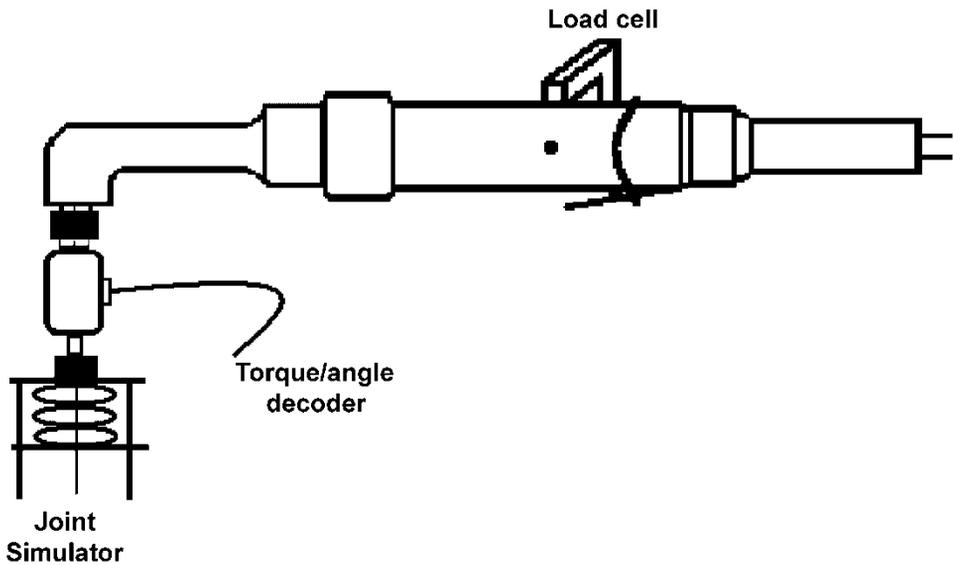
Figure 4. Diagram of the experimental arrangement. The tool was rigidly fixed to a platform to minimize inertial effect.
