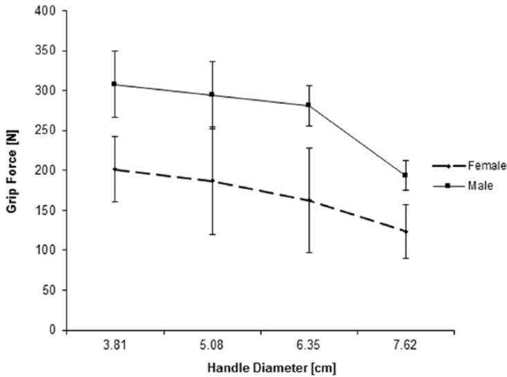
Figure 3. Maximal grip force vector magnitudes. Grip force magnitude decreases with handle diameter for both males and females.
