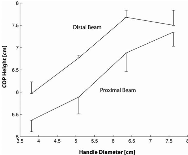
Figure 5. Vertical centers of pressure (COPs) versus handle diameter. Vertical centers of pressure generally increased with handle diameter for both instrumented beams.
