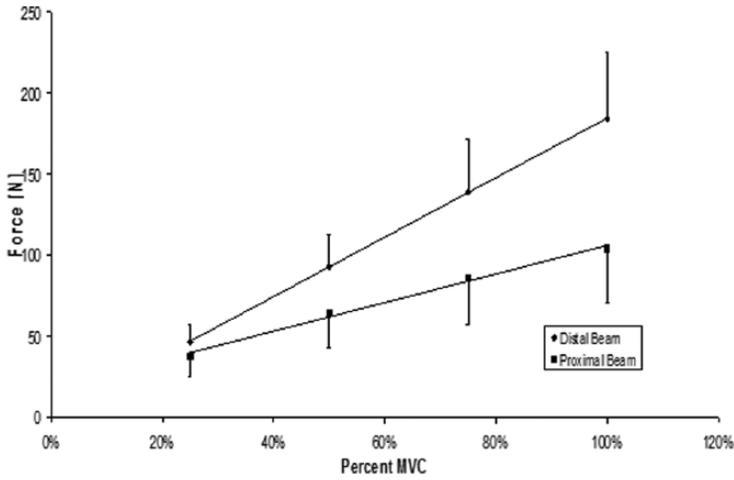
Figure 4. Scalar magnitude of the grip force vectors measured by each individual beam. The distal beam measured a larger portion of grip force applied by the fingers than the proximal beam. MVC = maximum voluntary contraction.
