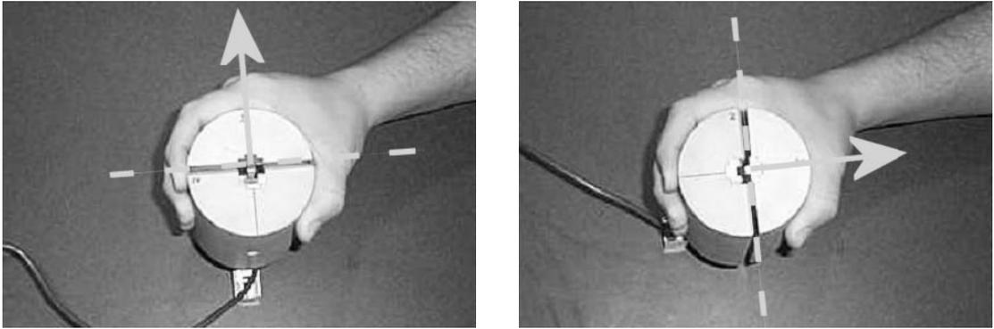
Figure 3. Procedure used for grasping the dynamometer. The handle was rotated 90° between trials in order to measure force in two orthogonal directions.
