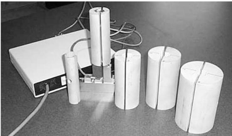
Figure 2. Dynamometer handle “caps” of varying sizes. Different caps were attached to the dynamometer in order to change the diameter of the cylindrical handle.
