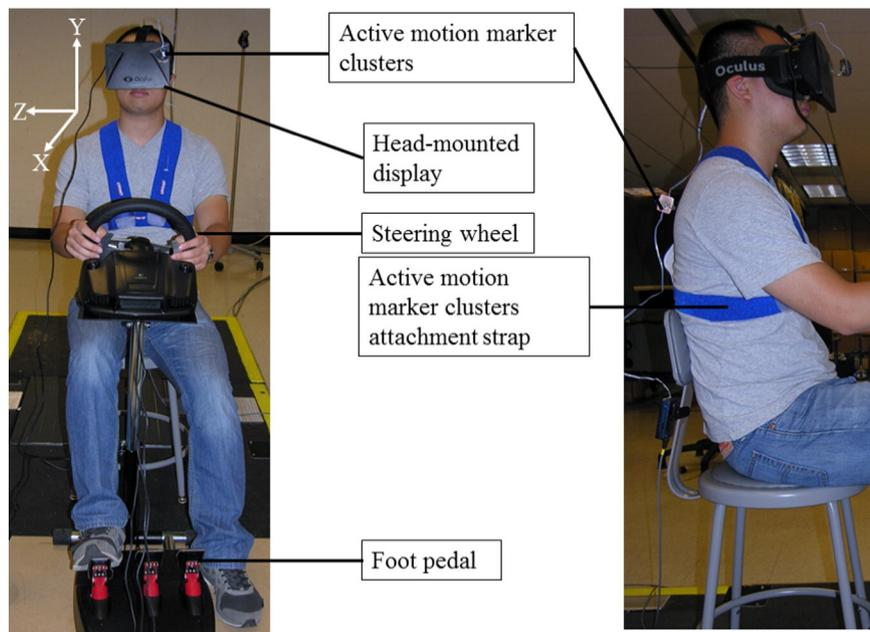
**Fig. 1.** A participant wore a head-mounted display and positioned the hands on a steering wheel, while the foot rested against one foot pedal. Active motion marker clusters were placed on the head-mounted display and on the trunk of the participant. The left image corresponds to the coordinate system indicated in the figure.
